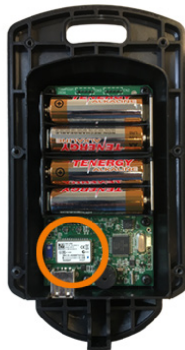
The Bluetooth module (circled) inside the Extreme Blue clock is a receiver and a transmitter.
