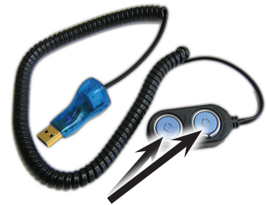
Blue Dot Receptor. You can touch your iButton to either of the two blue probes.
